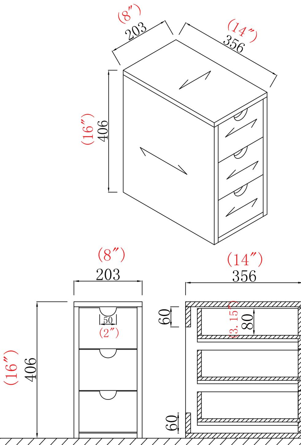
**ATTENTION!** Dimensions may vary by up to 3/8". It is highly recommended to pull all dimensions of actual model for installation and measuring purposes.
