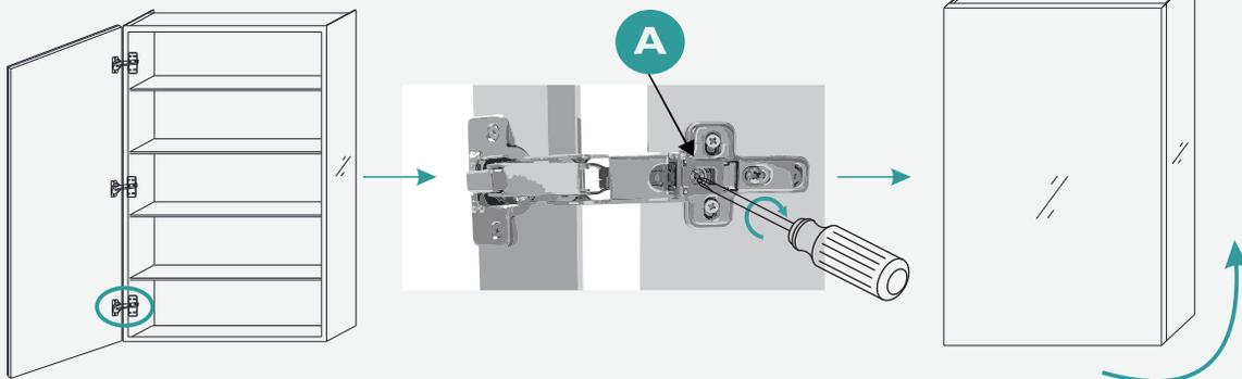
Find the top hinge and the screw **A** on hinge, turn the screw counter-clockwise, then the door will be turned down.
