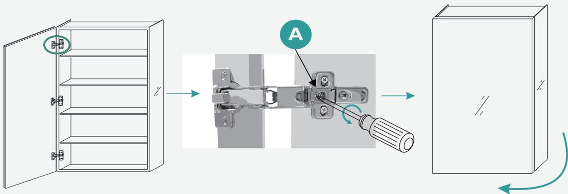
Find all hinges and the screw **B** on hinge, this screw allow you to adjust the distance between door and cabinet.
